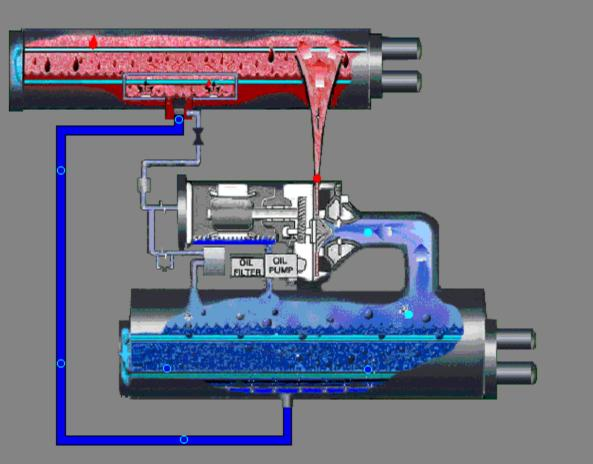
or refrigerant to ondense, it must be armer than *leaving* ondenser water.
