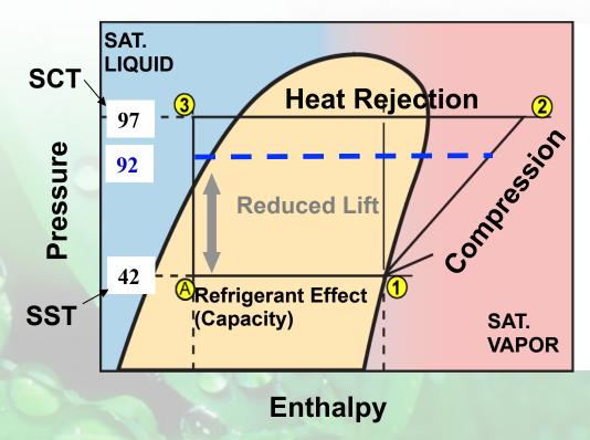
Lower Lift = Less Work = Lower kW
