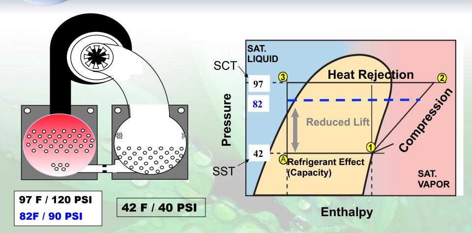
Lower Lift = Less Work = Lower kW
