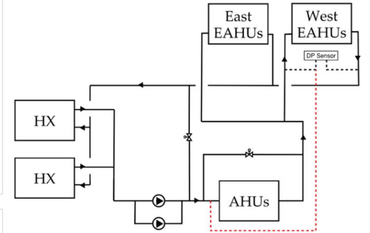
Building heat recovery loop schematic.
